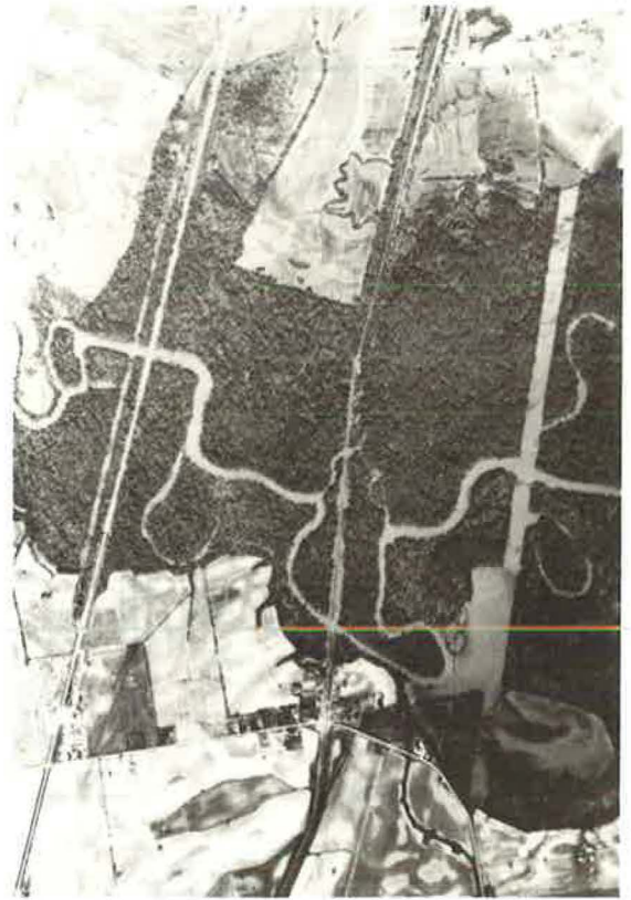
FIGURE 15 Aerial photograph, April 2, 1973 (channel Q = 9,218 \text{ ft}^3/\text{sec} , floodplain Q = 18,420 \text{ ft}^3/\text{sec} ).
