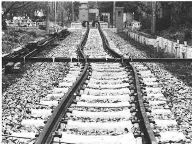
FIGURE 10 Full-scale test of track buckling.
