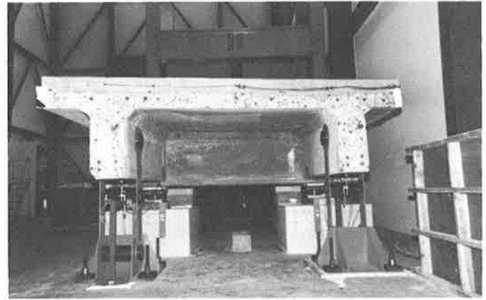
FIGURE 2 Gepford overhead bridge section laboratory setup
