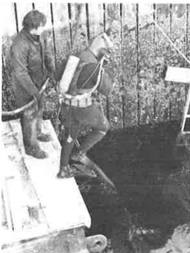
FIGURE 3 Diver ready for underwater inspections.
