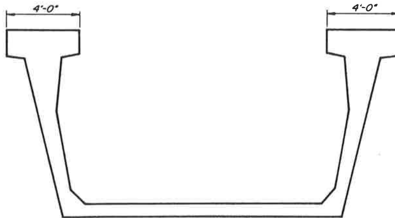
CROSS SECTION DURING DECK REPLACEMENT OPERATIONS
