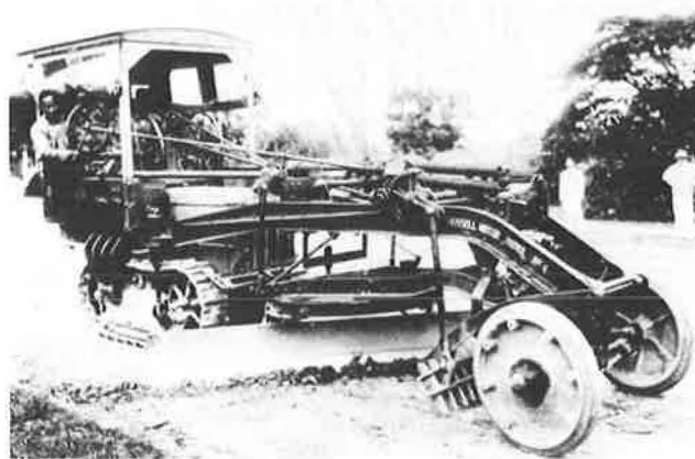
FIGURE 7 Prototype motorized grader, 1926.
