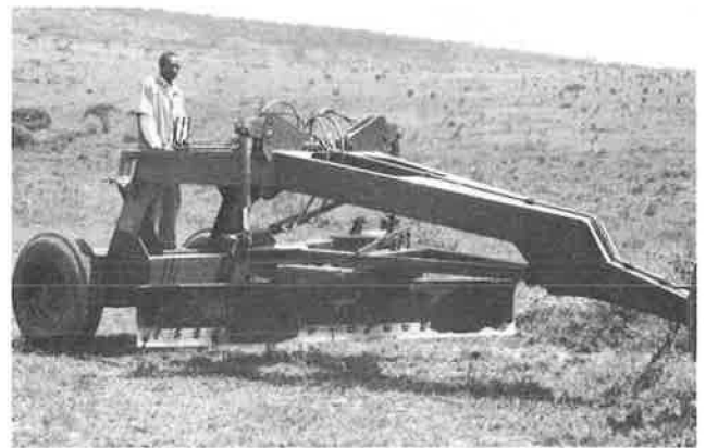
FIGURE 17 Prototype heavy grader on trial on clay soils.
