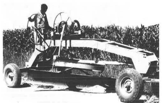
FIGURE 9 Towed grader currently utilized in Thailand.
