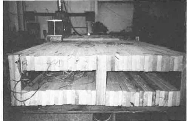
FIGURE 6 Stressed boxed-girder model at West Virginia University, 16-ft span with 2- by 6-in. top and bottom flanges with 3- by 16-in. webs, which are continuous through the top and bottom flanges.
