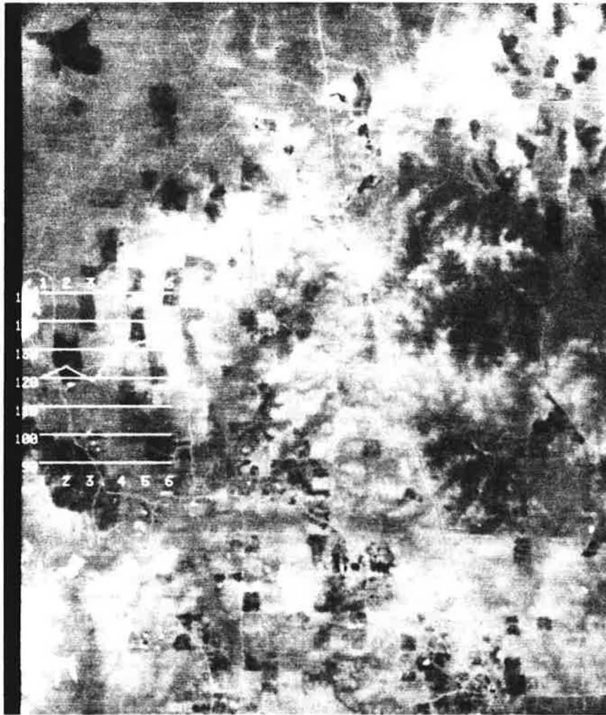
FIGURE 1 A TIMS thermal image of the Williana, La., area with a display of the spectral signature for the pixel under the cursor (white cross), produced with the SIXBP software program.
