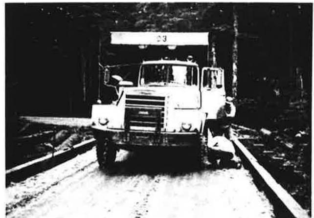
FIGURE 9 Bridge deck used for setting pressures and deflections.
