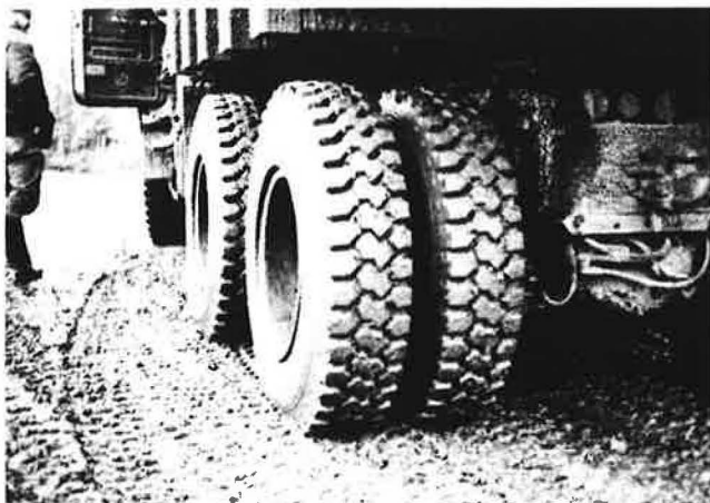
FIGURE 8 Mounted 12.00R24 radial tires.
