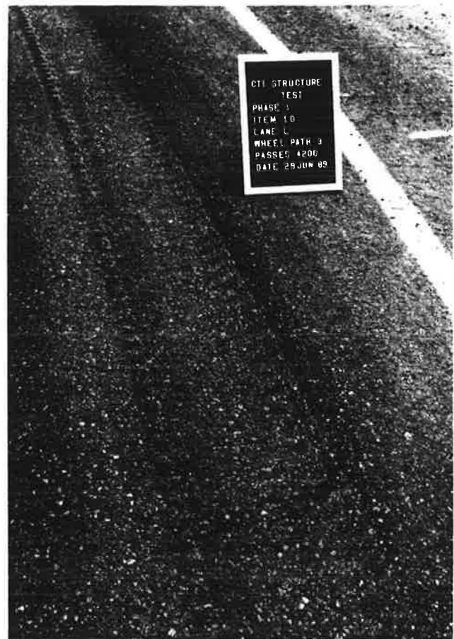
FIGURE 8 Low-pressure lane, Section 10, low-severity shoving after 4,200 passes.
