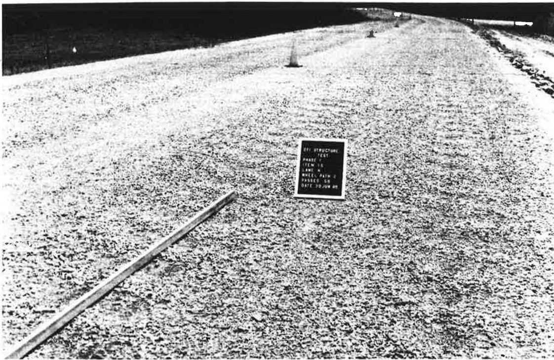
FIGURE 11 High-pressure lane, Section 15, low-severity washboarding, after 58 passes.
