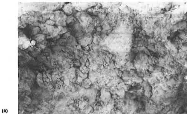
FIGURE 5 Scanning electron micrograph of Soil A with (a) 0 percent, (b) 3 percent, (c) 6 percent, and (d) 9 percent lime, cured for 28 days. (Magnification: \times 96 )
