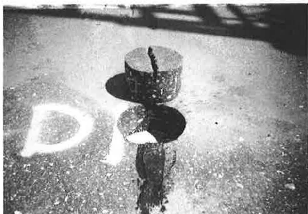
FIGURE 7 Core of transverse crack taken from low side of superelevated curve in Section 2.
