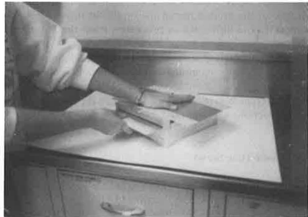
FIGURE 7 Metal plate being pulled out so that chips fall evenly onto binder surface.
