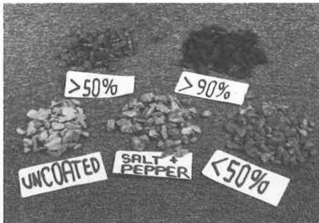
FIGURE 1 Typical five precoating conditions.
