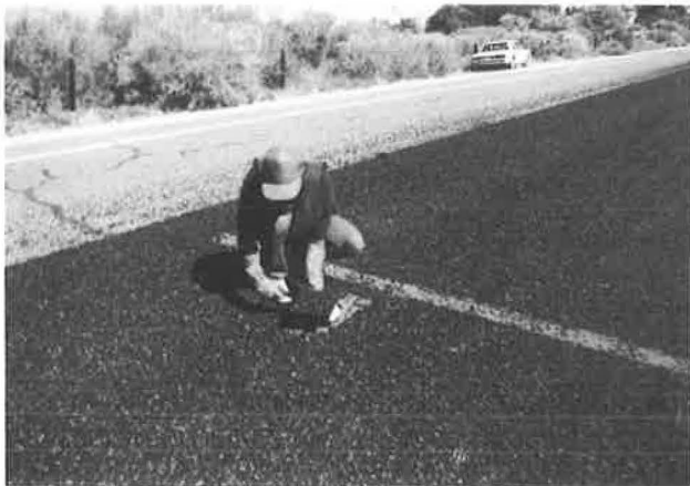
FIGURE 2 Removal of Vialit plates for testing.
