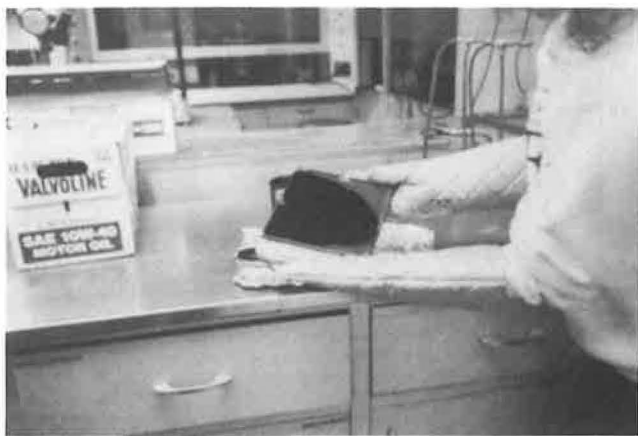
FIGURE 4 Preparation of sample plate (application of binder).
