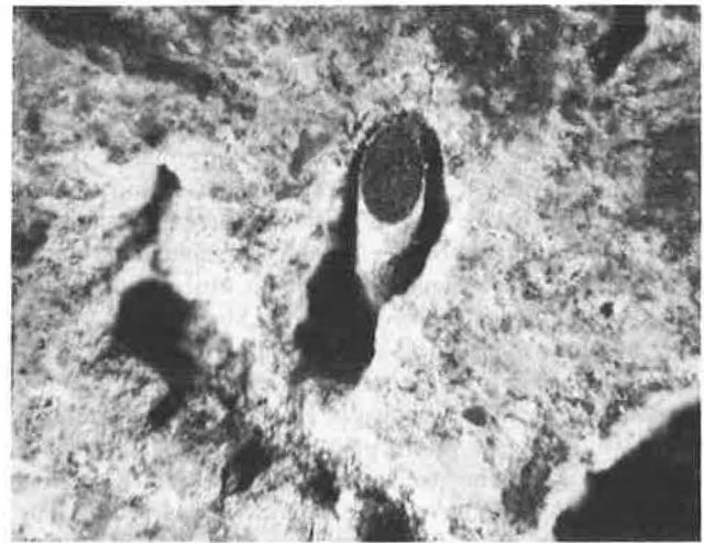
FIGURE 15 Typical fiber interface microcracks.
