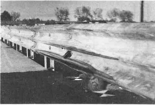
FIGURE 16 Vehicle contact marks, Test 476.
