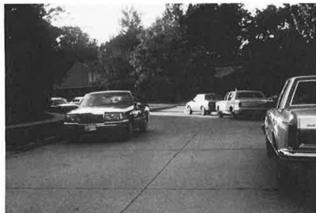
FIGURE 1 Parked cars and vegetation limit sight distance.
