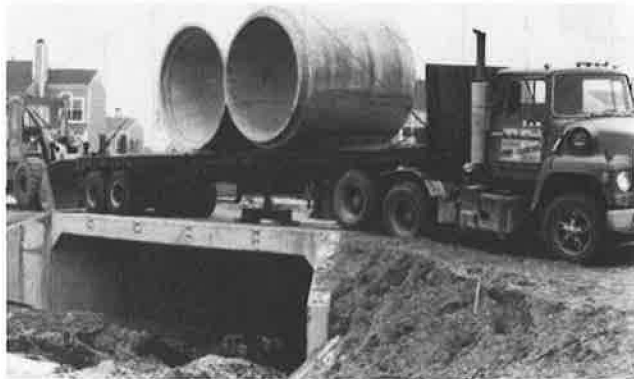
FIGURE 4 Load-deflection test arrangement for three-sided bridge.
