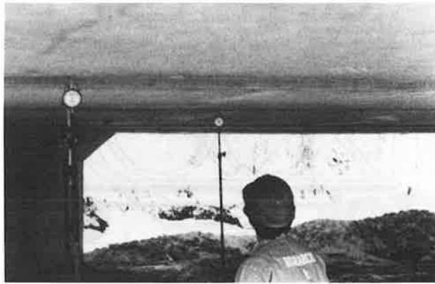
FIGURE 6 Deflections were obtained by three dial indicators. Locations relative to the load points are indicated in Figures 1, 2, and 7.
