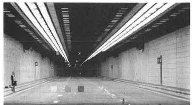
FIGURE 4 Targets at night under symmetrical lighting system.
