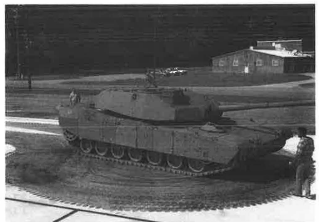
FIGURE 6 M-1 tank performing pivot steer turns on RMP test strip.
