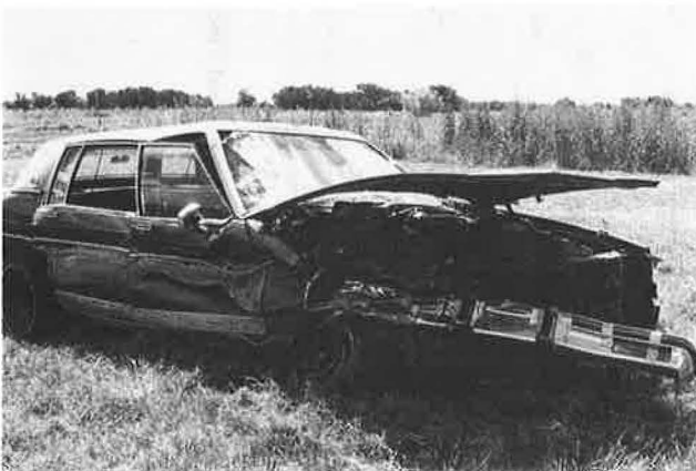
FIGURE 9 Oldsmobile before and after impact with T421 bridge rail.
