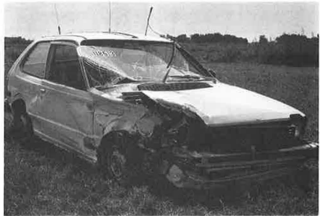
FIGURE 7 Honda before and after impact with T421 bridge rail.
