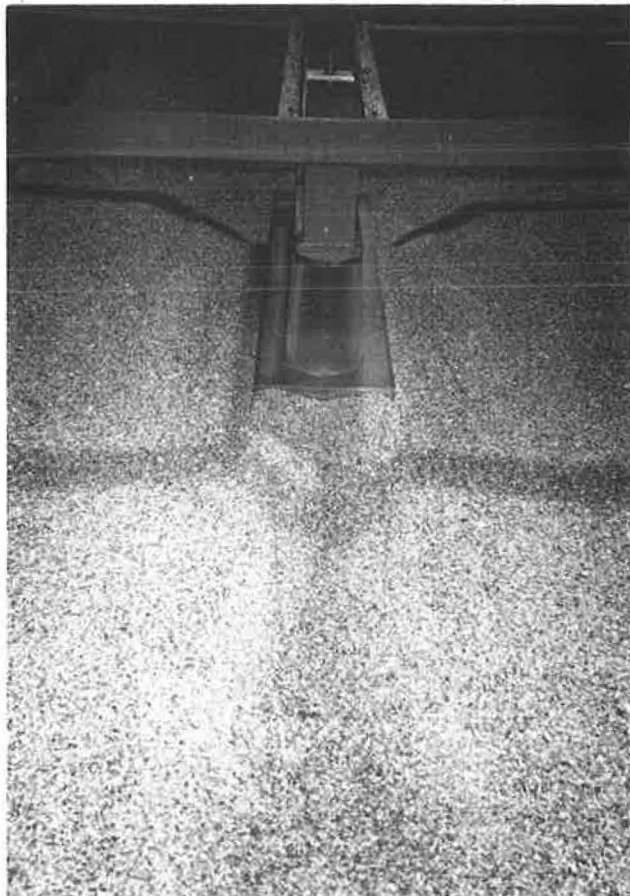
FIGURE 6 Scour alongside the aligned pier (Run 3).
