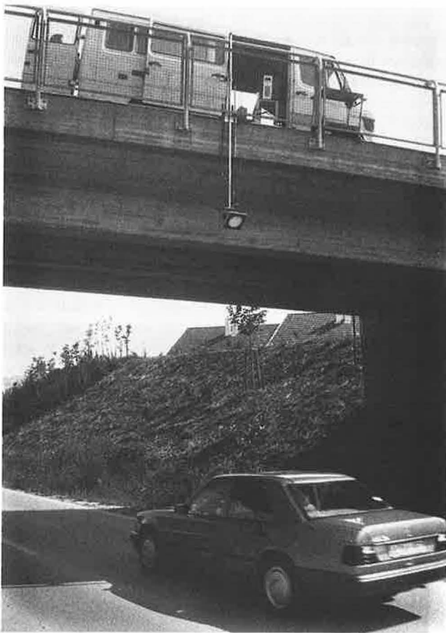
FIGURE 11 Measurement test setup for radar signature recording with parallel video recording. Small size and easy ambulant installation of the millimeter-wave radar detector are clearly recognizable.
