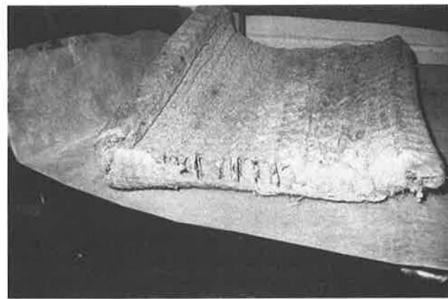
FIGURE 4 Geocomposite completely plugged by fines from I-65 in Kentucky.
