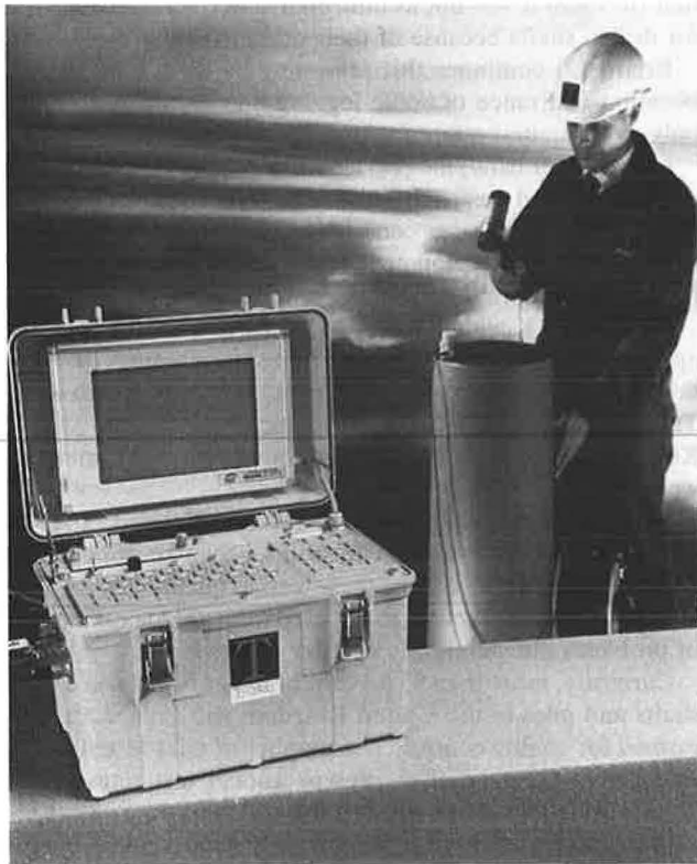
FIGURE 1 MIMP 15 integrity testing equipment with transducers shown on pile.
