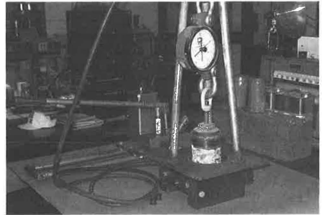
FIGURE 4 Cores of bonded overlay pull tested in laboratory.
