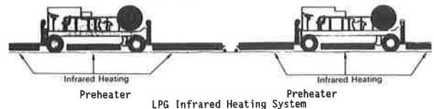
GENERAL VIEW OF HEAT REFORMING PROCESS (HRP-5) AT SPOKANE INTERNATIONAL AIRPORT SHOWING THE TWO PREHEATERS AND REFORMER. The pre-milled (75 mm) keel section involved heater scarification/rejuvenation (50 mm) with new surface course placement (50 mm) in one pass (Remix-Repave Option) [6].
