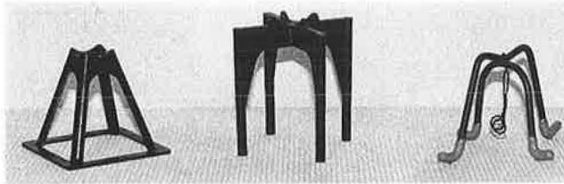
FIGURE 10 Rebar support chairs approved for Florida use. Left , polystyrene foam—1,000-lb capacity; middle , another producer's chair made from polycarbonate/ABS; and right , conventional chair made from steel that rusts.
