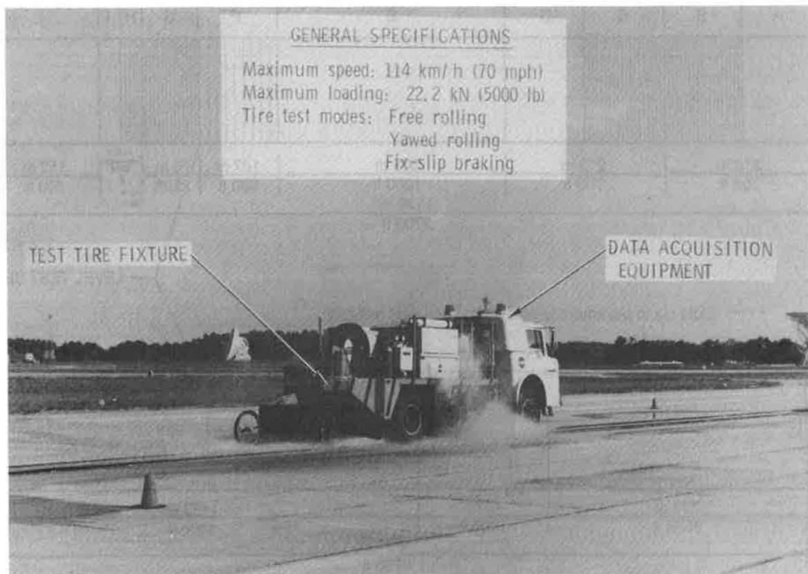
FIGURE 5 Instrumented tire test vehicle.
