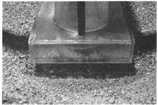
FIGURE 6 Vertically supported falling rod installed through pier footing.
