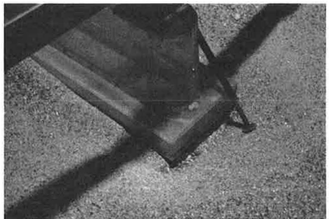
FIGURE 7 Sounding rod with base plate installed at 45 degrees from horizontal.
