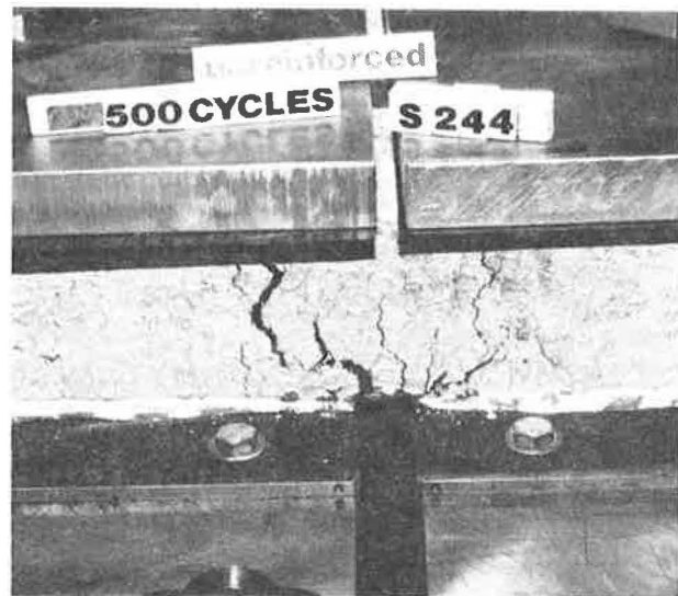
FIGURE 10 Failure mode-cracking pattern for unreinforced AC slab during combined tensile and shear stress test.
