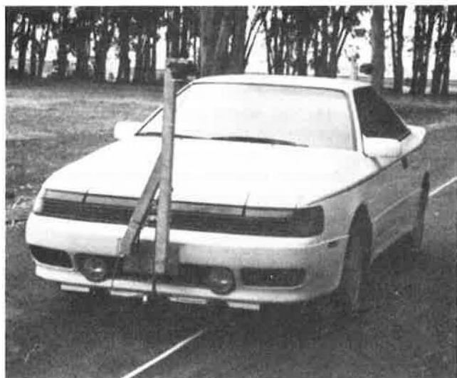
FIGURE 5 Experimental vehicle with independent measurement system.
