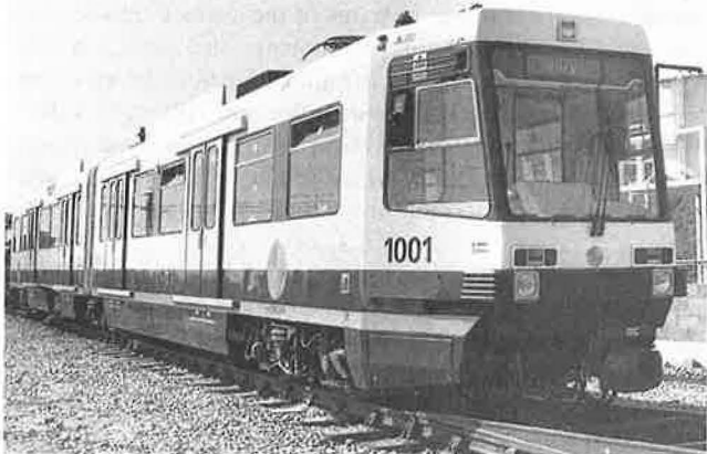
FIGURE 1 A six-axle articulated LRV built for Metrolink by Firema in Italy with electrical equipment by GEC Alstom.
