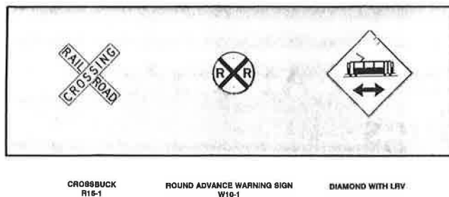
FIGURE 1 LRT grade crossing warning signs.
