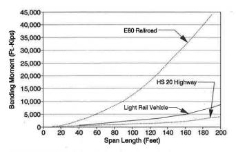
FIGURE 1 Vehicle bending moments on simple spans.
