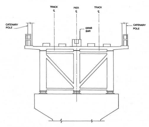
FIGURE 10 Typical section, steel girder span.
