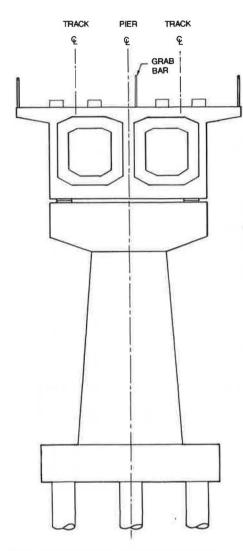
FIGURE 12 Typical section, concrete segmental bridge.
