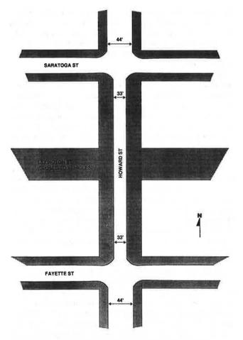
FIGURE 6 Curb and sidewalk configuration in the Lexington Mall area.
