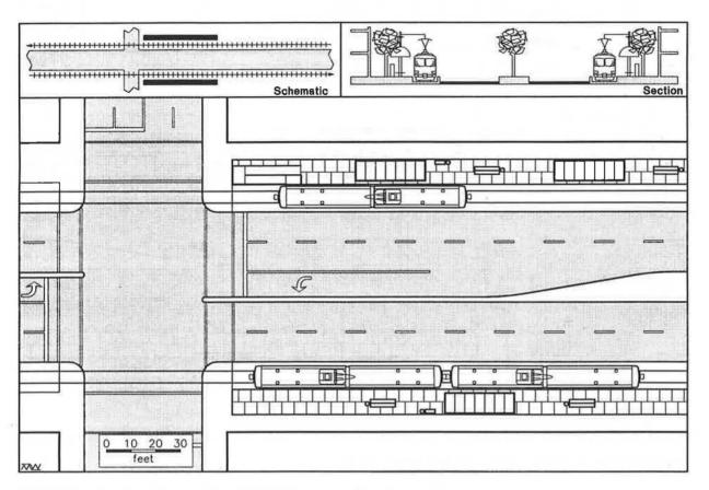
FIGURE 5 Sidewalk platform station with LRT along both sides of the street.
