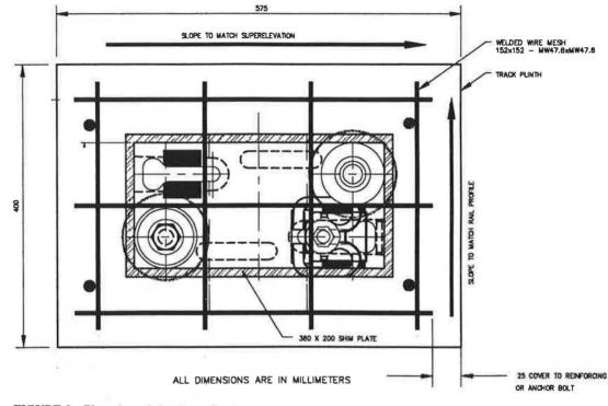
FIGURE 2 Plan view of the direct fixation assembly.
