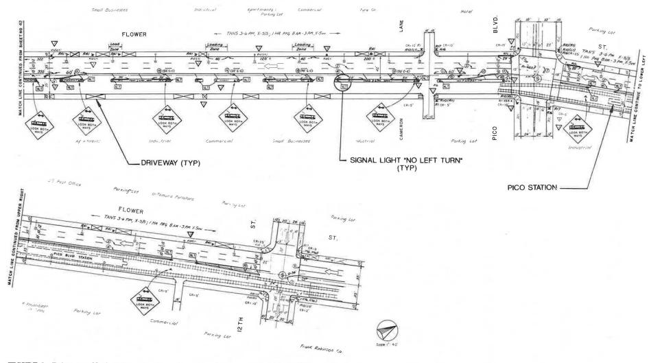
FIGURE 3 Driveways, No Left Turn signals, and warning signs on a typical block of Flower Street.
