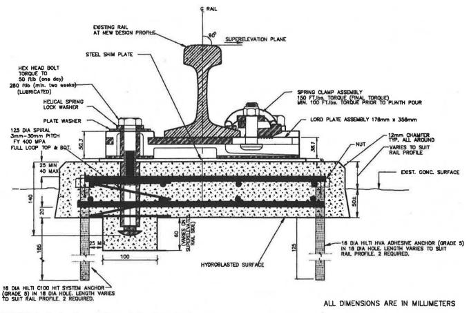
FIGURE 3 Section through the south line direct fixation assembly.
