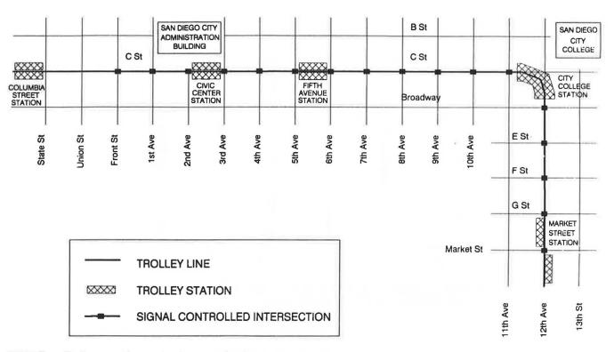
FIGURE 1 Trolley operation on signalized arterials in downtown San Diego.
