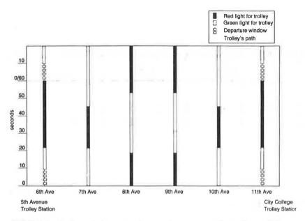
FIGURE 2 Trolley priority system (progressive movement for trolley on C Street between Fifth Avenue and City College Stations).
