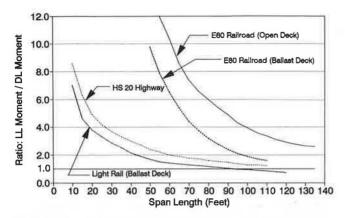
FIGURE 4 Typical bridge live-load-to-dead-load ratios.
