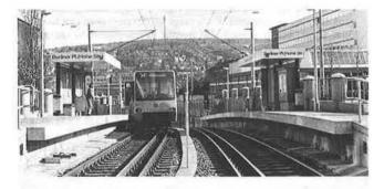
FIGURE 5 Three-rail track for mixed operation.
