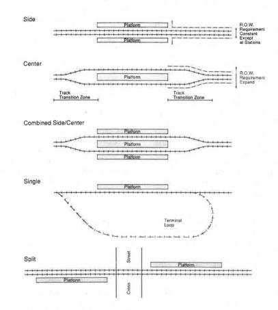
FIGURE 3 LRT platform configurations.
