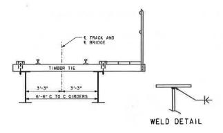
FIGURE 2 Section through open deck bridge and weld detail.
