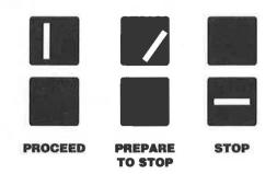
FIGURE 8 The three aspects of the positioned bar LRT signals.
