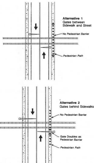
FIGURE 4 LRT gates at midblock crossings.
