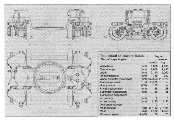
FIGURE 1 Unpowered truck on Bern low-floor car.
