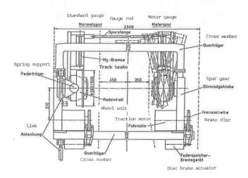
FIGURE 6 Diagram of single-wheel running gear of VÖV low-floor car.
