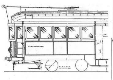
FIGURE 2 Schematic drawings of the Melbourne Class W-2 streetcar.
