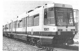
FIGURE 1 A six-axle articulated LRV built for Metrolink by Firema in Italy with electrical equipment by GEC Alsthom.
