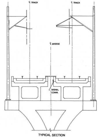
FIGURE 18 Typical pole mounting details on piers: ballast
