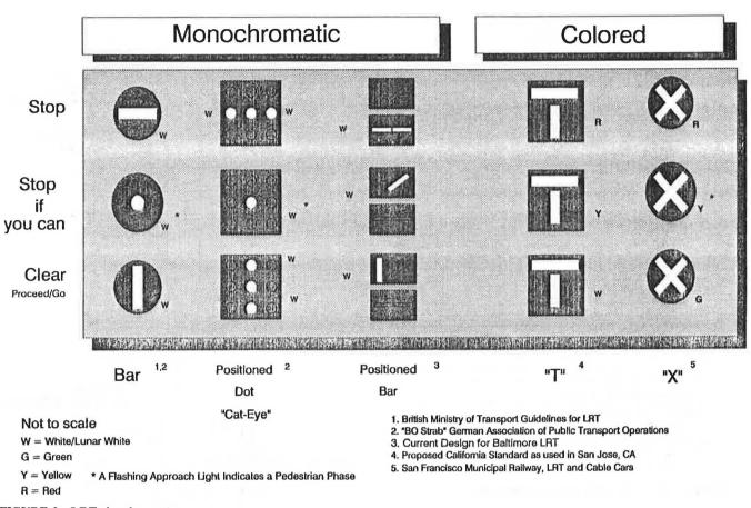
FIGURE 2 LRT signal aspects.
