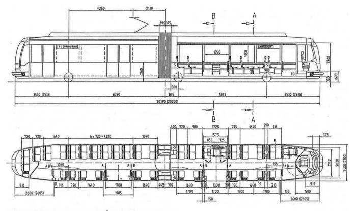
FIGURE 4 Principal dimensions of VÖV two-section low-floor car.
