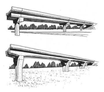
FIGURE 1 Metro Link bridge: (top) preliminary engineering phase—post and lintel bridge with constant depth beam on hammerhead piers; (bottom) final design—cast-in-place slingshot piers with haunched beamed curved superstructure.
