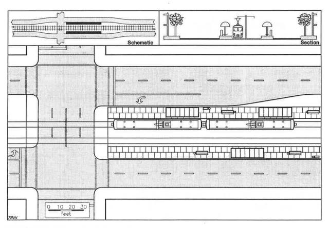
FIGURE 2 Side platform station in street median.
