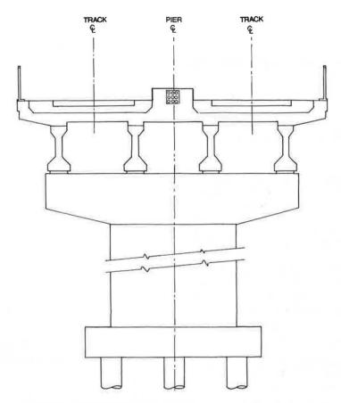
FIGURE 9 Typical section, AASHTO beam span ballast deck.
