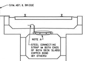
NOTE A: ALL LAPS SHALL BE TACK WELDED TO MAKE REINFORCEMENT ELECTRICALLY CONTINUOUS THROUGHOUT LENGTH OF EACH DECK SECTION. AT BOTH ENDS OF EACH DECK SECTION THESE 4 BARS SHOULD BE CONNECTED TOGETHER BY A 11/2" × 1/4" FLAT STEEL SECTION WELDED TO THE BARS AND BROUGHT TO THE SURFACE OF THE CONCRETE.
