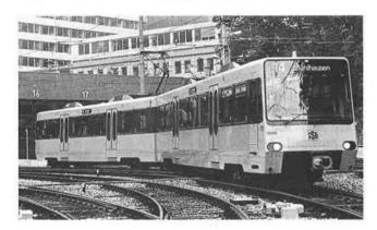
FIGURE 4 A two-unit Stuttgart LRV (Type DT8).
