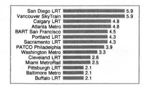
FIGURE 8 Energy efficiency in passenger miles per kilowatt hour of electricity.
