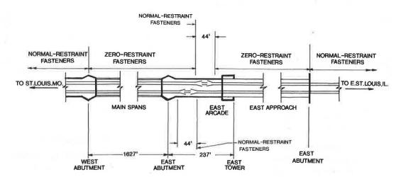
FIGURE 16 Typical rail expansion joint configuration.
