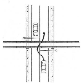
FIGURE 6 Automobile driving around lowered crossing gates.
