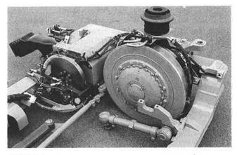
FIGURE 5 Powered single-wheel running gear of VÖV low-floor car.
