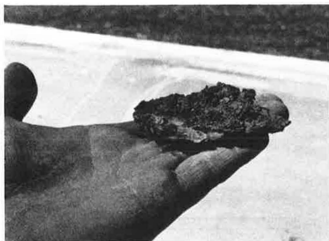
FIGURE 4 Ice lens removed from frost-susceptible silty subgrade at about 1.5 m. This excavation work was completed in late July after normal summer weather in the District Municipality of Muskoka.
