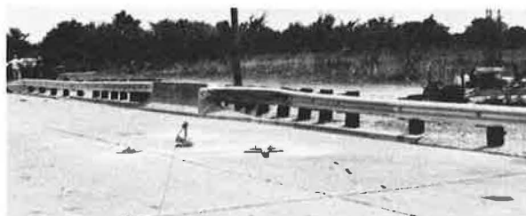
FIGURE 2 Integral end-post transition after Test 1.
