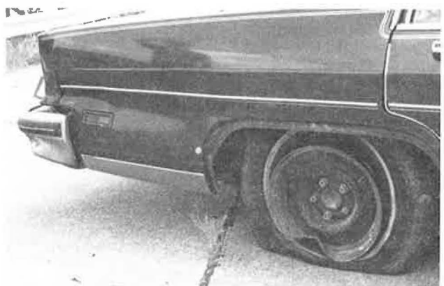
FIGURE 9 Photographs of damage to vehicle after Test 7147-5.
