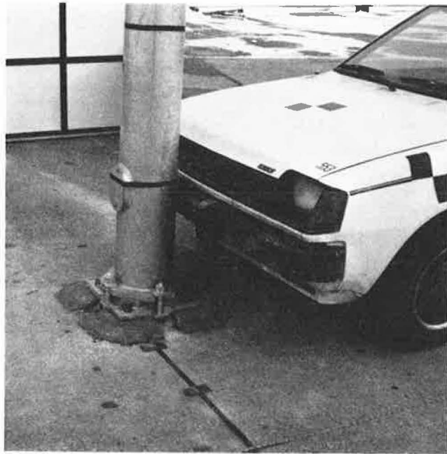
FIGURE 2 4-bolt breakaway slipbase installation.
