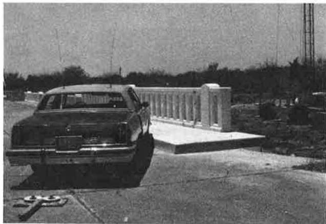
FIGURE 14 Vehicle and bridge rail installation geometrics for Test 1185-6.
