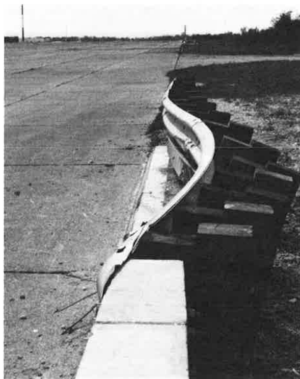
FIGURE 8 Improved separate end-post transition after improved design test.
