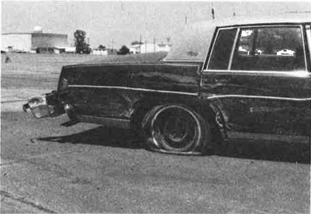
FIGURE 16 Damage to right side of vehicle, Test 1185-6.
