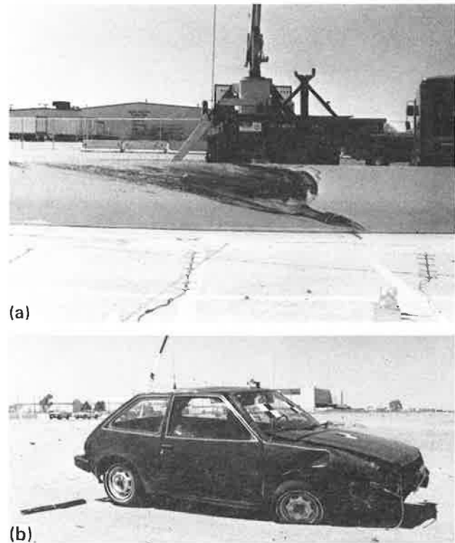
FIGURE 7 Damage to (a) bridge rail and (b) test vehicle, Test MS30-2.
