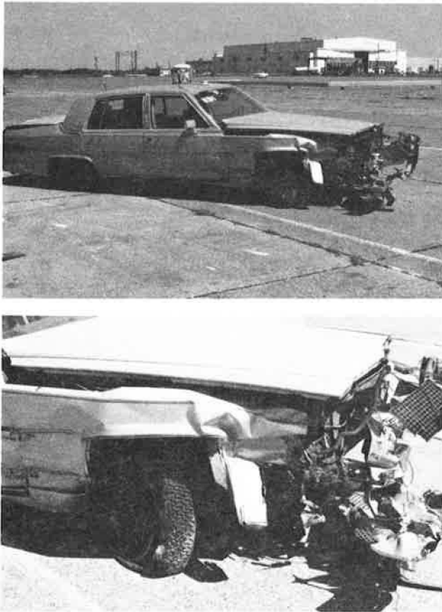
FIGURE 4 Photographs of damage to vehicle after Test 7147-2.
