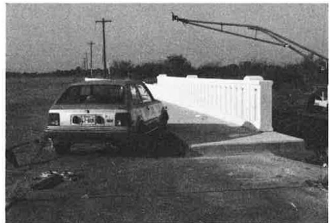
FIGURE 8 Vehicle and bridge rail installation geometrics for Test 1185-5.
