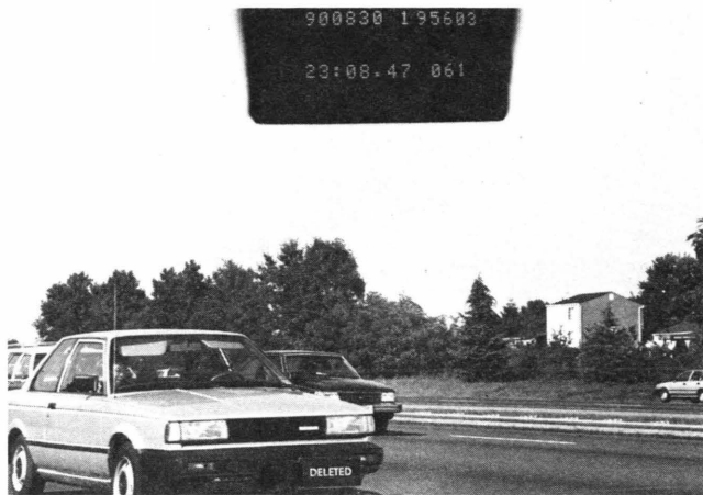
FIGURE 2 Typical photograph produced by a photo-radar unit. License plate number was deleted to ensure the privacy of the vehicle's owner.
