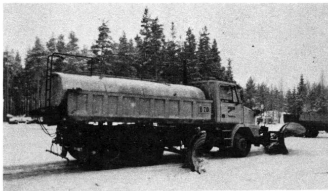
FIGURE 1 Finnish winter fighter with the plow, wing, and liquid salt spreader.
