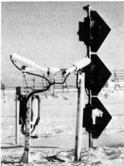
FIGURE 4 Field experiments for calibration of sensor against transmissometer.
