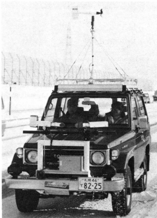
FIGURE 7 Sensor mounted on vehicle for observation; sampling area is set at 1.2 m height from road surface.
