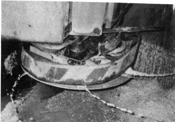
FIGURE 8 Spreader of Figure 7 seen from outside. Prewetted salt is dripping wet. Amount of prewetter is 20 weight percent.
