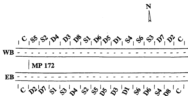
FIGURE 1 I-10 load transfer restoration test section layout.
