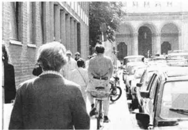
FIGURE 6 Service Level D: Schellingstrasse, Munich—pedestrian environment is visually boring, walled up on one side and parked cars on the other; cyclists and pedestrians are using same right of way, making it especially unsafe for captive groups.
