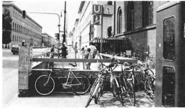
FIGURE 5 Service Level D: intersection of Leopoldstrasse and Schellingstrasse, Munich—effective walk width reduced by improper placement of street furniture and illegal bicycle parking; environment is hazardous for physically challenged pedestrians.
