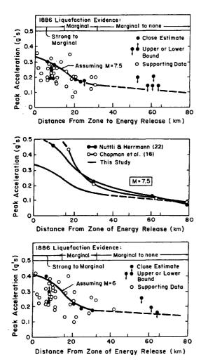
FIGURE 4 Top: Estimated attenuation of peak accelerations assuming 1886 event of M7.5; *middle:* comparison of attenuation curve from this study with curves proposed for eastern United States for M7.5 events; *bottom:* estimated attenuation of peak accelerations assuming 1886 event of M6.
