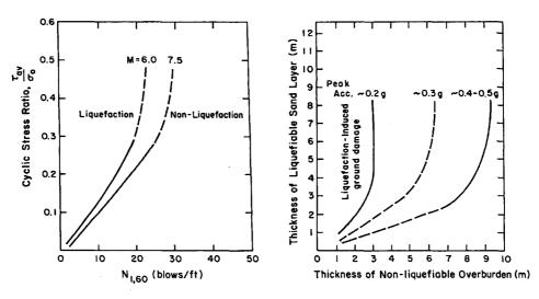
FIGURE 1 Left: SPT-based liquefaction prediction curves (4); right: boundary curves to predict surface disruption [modified from Ishihara (1)].
