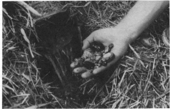
FIGURE 10 Gravel from punctured outlet pipe.
