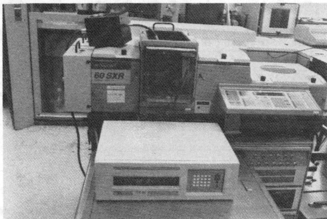
FIGURE 1 Minimat in Fourier transform infrared spectroscopy chamber.
