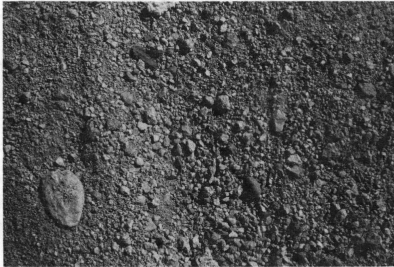
FIGURE 6 Representative texture and composition of excavated reinforced fill.
