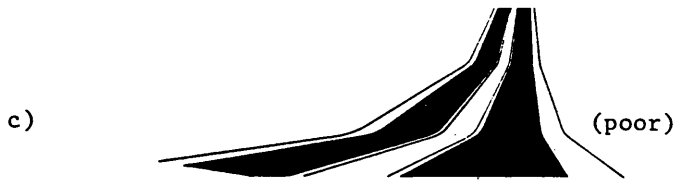
Broken-Back Vertical Curve
