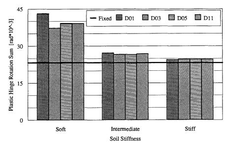
FIGURE 7 Comparison of instantaneous and cumulative column demands, higher intensity El Centro earthquake record, spread footing foundation.
