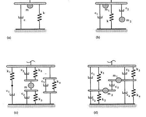
FIGURE 1 Discrete models of elastic half-space system: (a) 3 parameters, (b) 5 parameters, (c) 9 parameters, and (d) 11 parameters.
