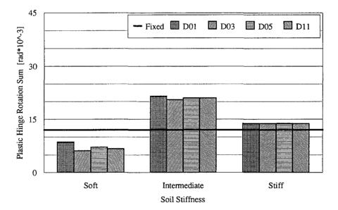
FIGURE 9 Comparison of instantaneous and cumulative column demands, higher intensity Olympia earthquake record, spread footing foundation.
