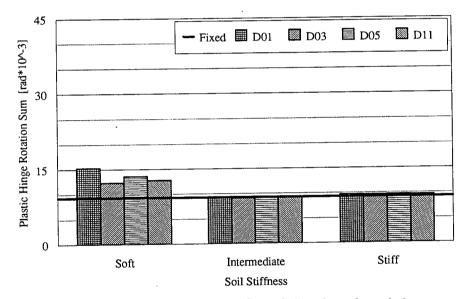
FIGURE 6 Comparison of instantaneous and cumulative column demands, lower intensity El Centro earthquake record, spread footing foundation.
