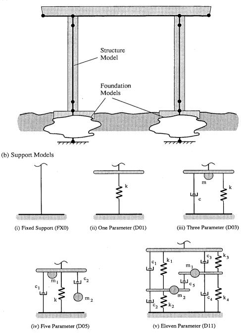
FIGURE 2 Schematic of NEABS models for the spread footing foundation study; (a) bent structure, and (b) foundation models.
