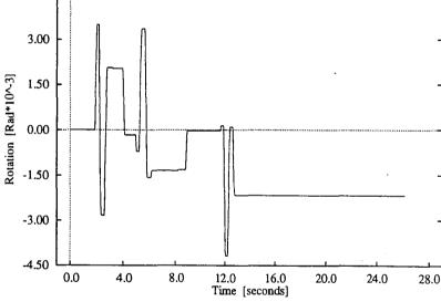
FIGURE 5 Typical hysteresis and plastic hinge rotation results.
