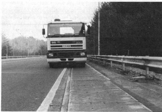
FIGURE 2 Load-measuring mat on TRL test track.
