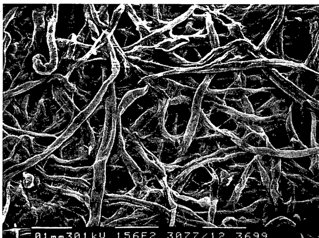
FIGURE 2 Scanning electron micrographs: left, Schleicher and Schuell No. 589 filter paper; right, Whatman filter paper.
