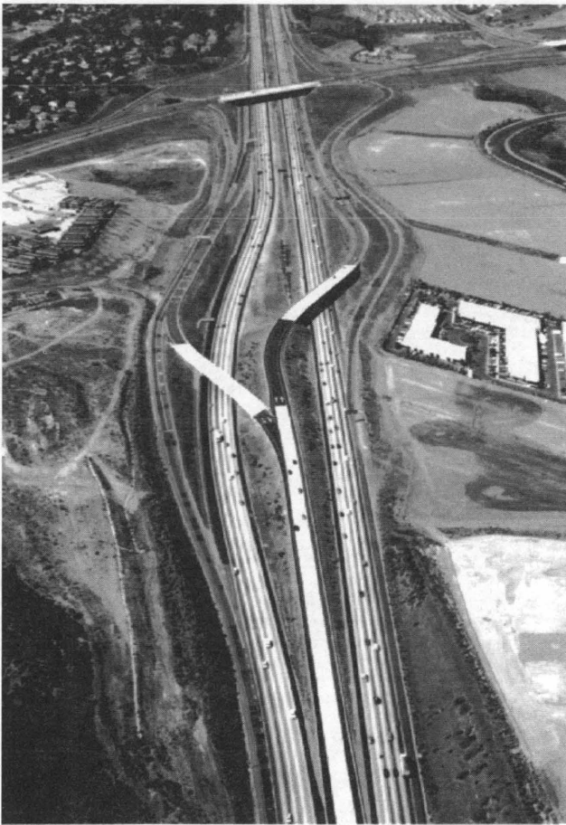
FIGURE 5 Direct connector ramps at northerly end of HOV facility. State Highway 56 interchange is at top.
