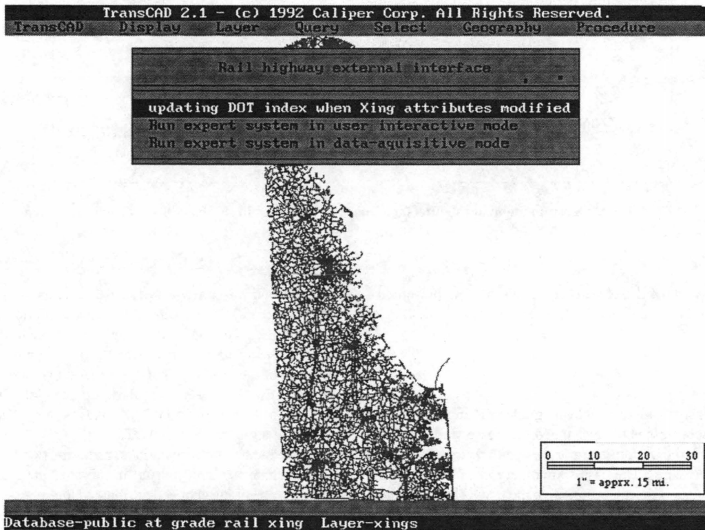
FIGURE 5 Interface menu for KBES in CLIPS and USDOT model from within TransCAD rail-highway application.
